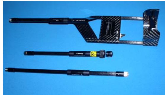
SnapOn Profiler head for a Pearpoint 494 camera/tractor unit
